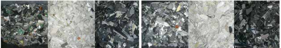
Figure 28. Post-separation plastics divided into brominated and non-brominated plastic using the Redwave XRF system. Source: Redwave Austria
