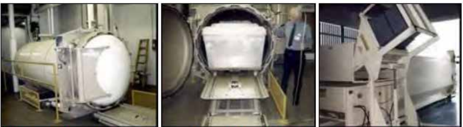
Figure 39. L-R: Bondtech autoclave, on-site autoclaev with lift table at a hospital, waste dumper.
