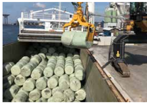
Figure 23. Baling and loading RDF in Ireland bound for Landskrona Energi Swedish Incinerator. Source: Geminor
