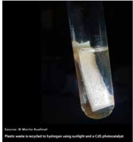
Figure 22. Photoreformation of plastic waste to hydrogen.
