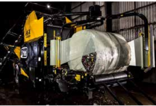
Figure 23. Baling and loading RDF in Ireland bound for Landskrona Energi Swedish Incinerator. Source: Geminor
