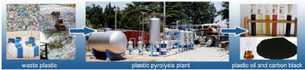
Figure 20. Plastic to fossil fuel via pyrolysis.
