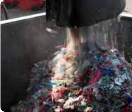
Figure 40b. Disinfected, shredded waste output from a Sanitech unit.
