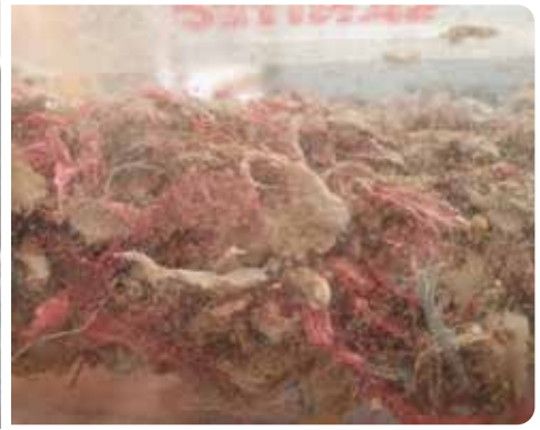
Figure 40b. Disinfected, shredded waste output from a Sanitech unit.
